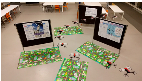
Fig. 7. Drone avoiding obstacles in the cafeteria experiment (9/10 successful flights).
